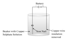
2. a) In the circuit given in the figure, Boojho observed that copper is deposited on the electrode connected to the negative terminal of the battery. Paheli tried to repeat the same experiment. But she could find only one copper plate. Therefore, she took a carbon rod as the negative electrode. Will copper still be deposited on the carbon rod? Explain your answer.
