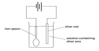
Silver ion is positively charged, so the spoon must be connected to a negative terminal to deposit silver on it. The other electrode should be made of silver.]
